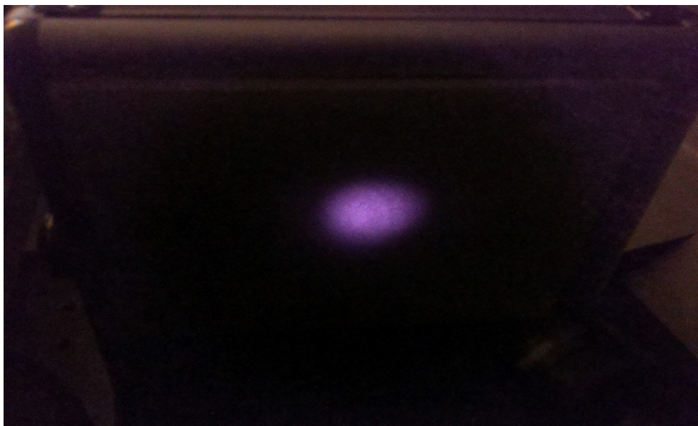
Fig. 10: Image taken using the above set-up. The lens spreads out the beam to make internal structure more visible. Even after multiple reflections the beam is powerful enough to saturate the camera.
