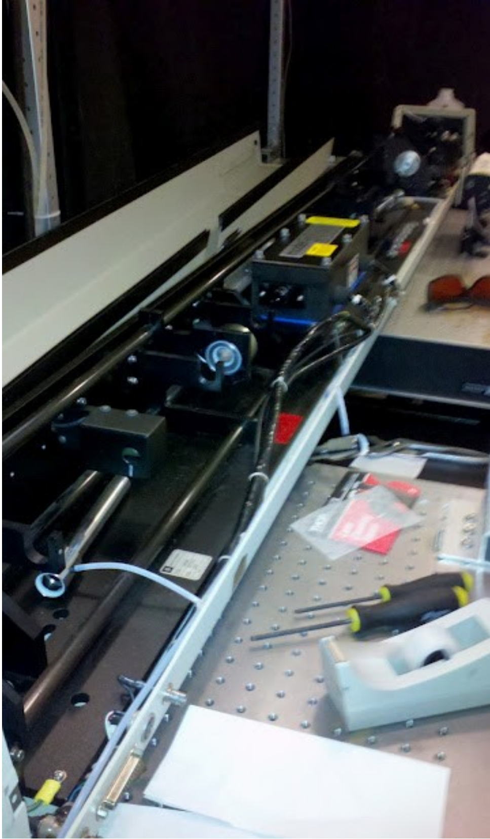
Fig. 6: The laser cavity. The lamp and rod are encased in the central box.
